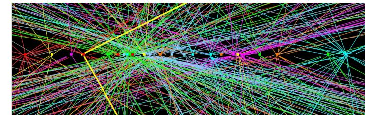
$Z \rightarrow \mu\mu$  with 25 reconstructed interaction vertices
