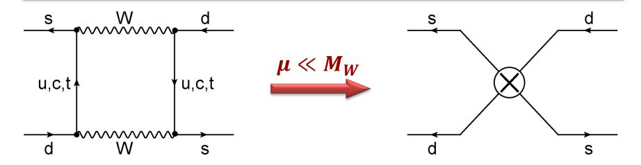
Integrating out W, the box diagram can be replaced by the local, four-quark operator
