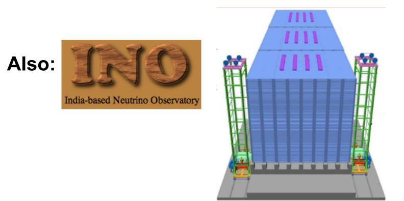
Focus on atmospheric neutrinos w/magnetized 50 kt iron calorimeter ICAL (get charge sign, nu vs nubar);
